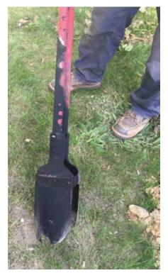
TIP: Always dig safely by using hand tools or soft excavation techniques within 24" of the marked infrastructure (make sure to check your state laws).
